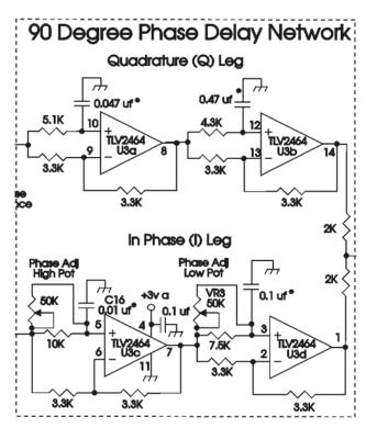
Figure 131. Audio phasing section schematic
