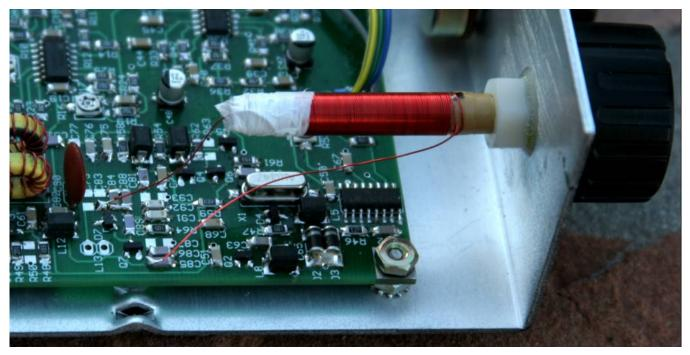
Figure 72. Main tuning PTO coil L13 shown mounted to the front panel. This is used only when the rig is finished.
