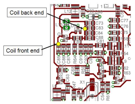
Figure 117. Connections for the PTO coil L13.
