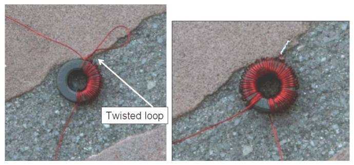
Figure 18. L2 details. After first 24 turns, add a twisted loop for later center tap. Add 27 more turns after this.
