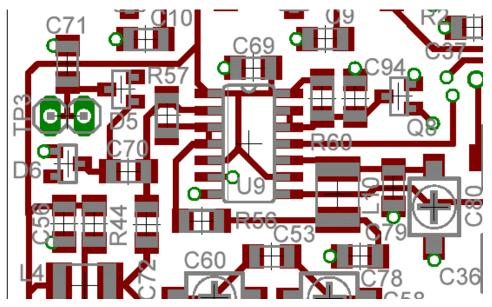
Figure 62. Close up view of the AFA RF Buffer and Phase Splitter Area
