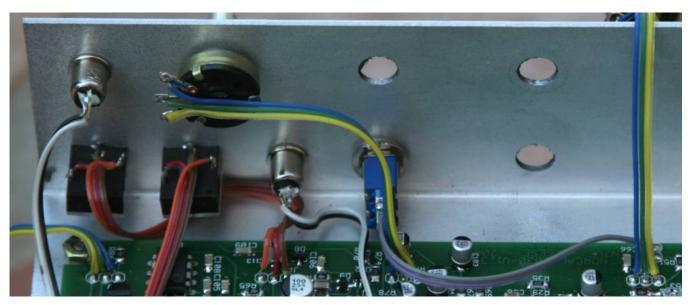
Figure 106. Mount the volume control pot (upper right) and the spot switch (lower middle).
