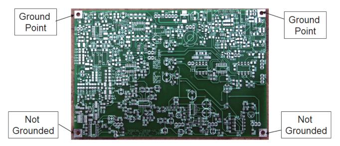
Figure 31. Ground reference for voltage measurements are upper 2 corners, the lower 2 are not connected
