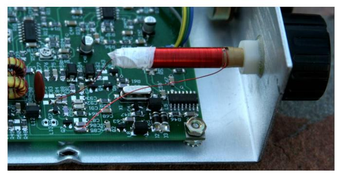
Figure 116. PTO L13 mounting detail. Coil connections shown. Front PTO coil wire must connect as shown.
