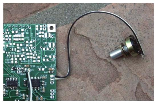
Figure 46. Connect R88 CW speed pot to the R88 pads as shown. Keep black and white in order shown.
