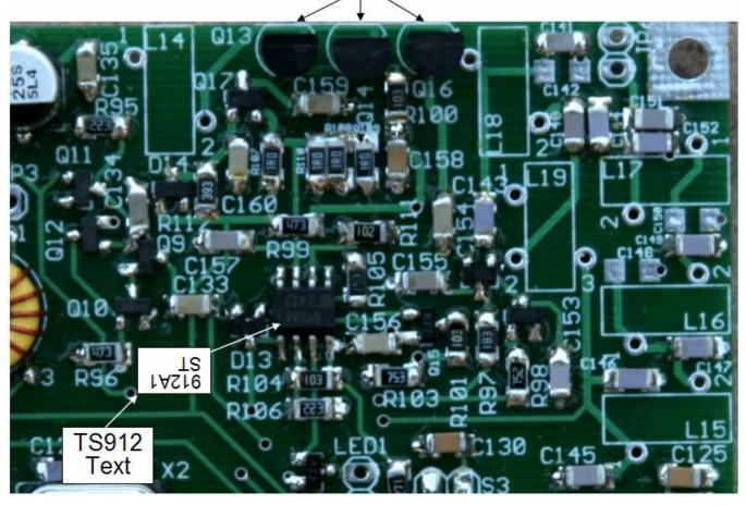
Figure 96. All transmitter parts except for the inductors. Note TS912 orientation, BS170 flat side orientation.
