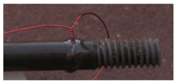
Figure 74. First turn is glued (epoxy) into place to make it easier to wrap the rest of the turns
