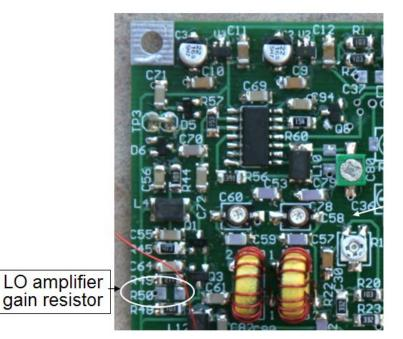
Figure 125. Location of optional LO amplifier gain adjust resistor R50
