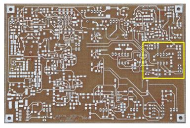
Figure 38. Location of the CW Keyer section of the board
