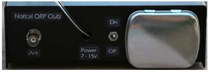
Figure 113. Placement of the switching supply tin on the back chassis, power jack not installed.
