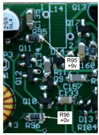
Figure 100. Location of R95 and R96. Voltages on transmit/receive switches
