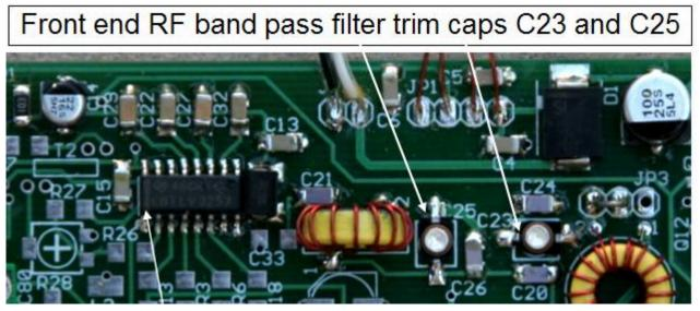
Figure 126. Location of RF front end band pass filter adjust trim caps, C23 and C25 on top middle of the board
