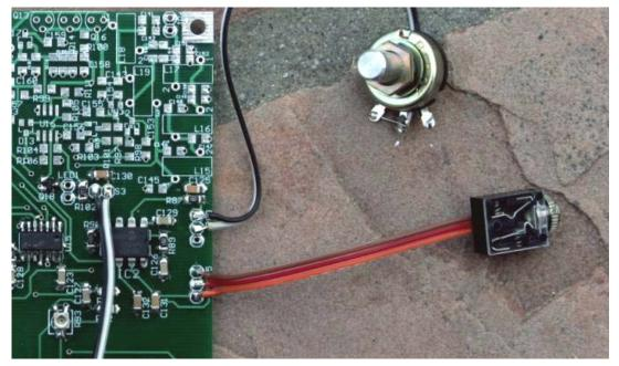
Figure 48. Attach paddle jack to JP5 using the color order shown
