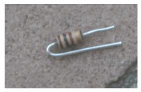
Figure 20. 100 ohm Temporary 3v Load Resistor Formed as Shown
