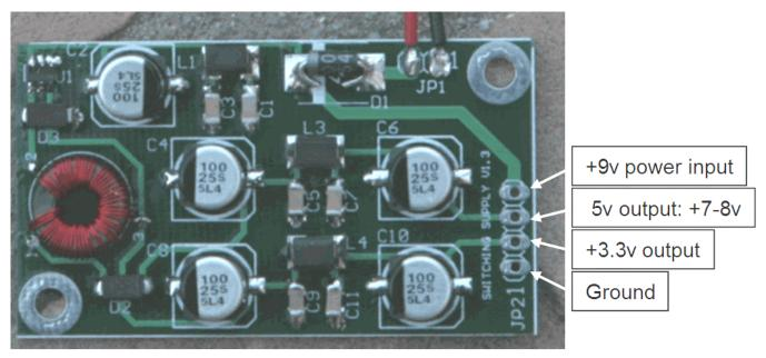
Figure 23. Power Output Connection Details (Load resistor not shown)
