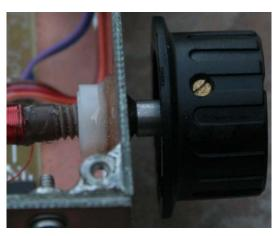
Figure 120. PTO brass screw full inserted into the PTO coil
