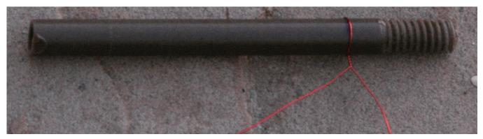
Figure 73. Wrap first turn on the PTO coil. Position <sup>3</sup>/<sub>4</sub>" back from front, twist single turn in place
