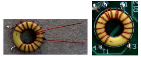
Figure 86. Detail on T1. Two turn # 32 to pads 1 & 2. Main winding connect to pads 3 & 4.
