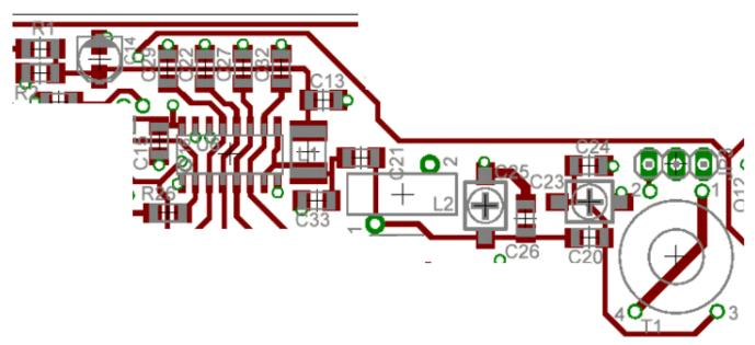
Figure 84. Close up of the detector and the RF tuned front end
