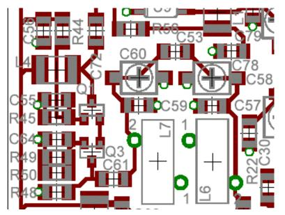
Figure 80. Close up of the LO Filter and Amp components
