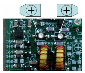
Figure 81. LO Filter and amplifier as built. Both trim caps must have proper orientation
