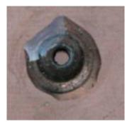
Figure 118. Front side of the PTO coil (prototype chassis) showing epoxy ridge from the front side
