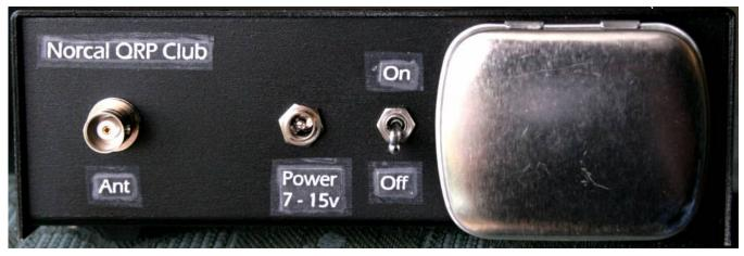
Figure 109. Rear panel of prototype NC2030. Final case will be silk screened.
