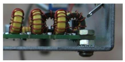
Figure 101. Mount all four corners of the main board using the mounting hardware as shown.
