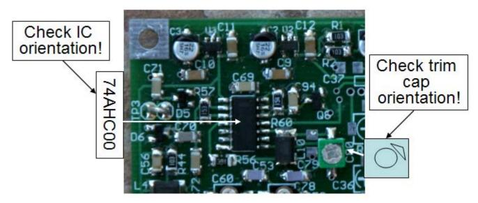
Figure 63. Orientation of U9 labeling as installed.
