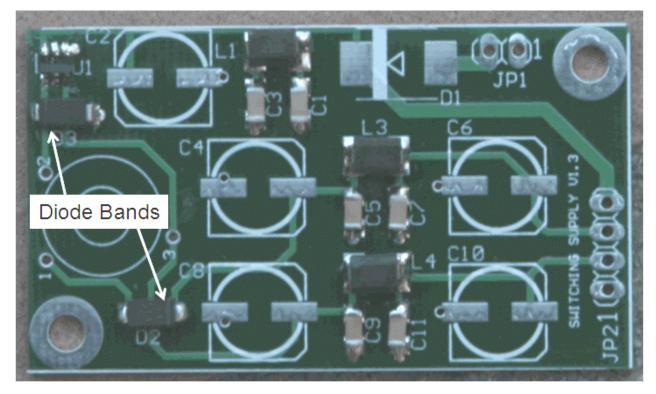
Figure 15. PS with 0.1 Caps, 47 uH inductors, Schottky diodes, and Switching IC
