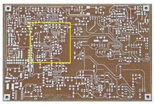
Figure 88. Location of Audio Preamp and Phasing sections
