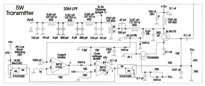
Figure 139. Schematic of Class E Transmitter
