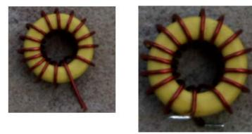
Figure 87. L2 leads formed to prepare for surface mounting on the top of the through hole pads provided.
