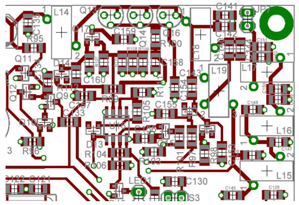
Figure 95. Close up of the transmitter section portion
