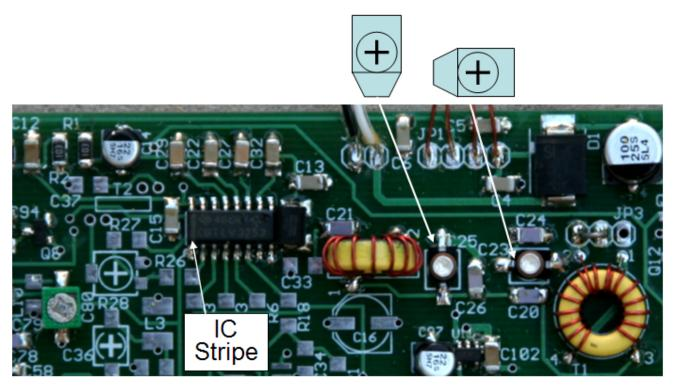
Figure 85. Picture of detector and RF front end with parts installed. Note trim cap orientation and jumper on JP3!
