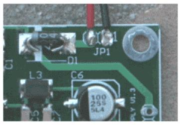
Figure 21. 1N4001 Mounted and 9v Battery Clip Connected
