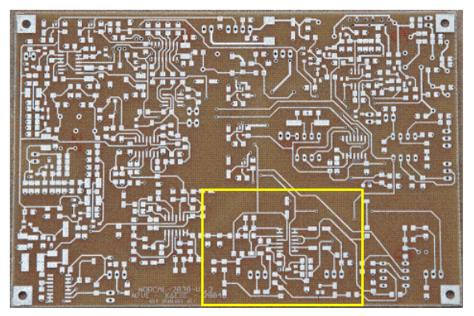
Figure 32. SCAF, HPF, Audio Amp, and Headphone driver section of the board
