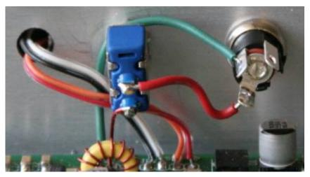
Figure 112. Power jack connections, +12v to power switch (red wire) and ground (green) to JP2 ground pad
