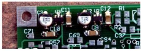
Figure 28. Parts layout of first two 2.9v LDO regulators. Note the black band orientation of the electrolytic caps.
