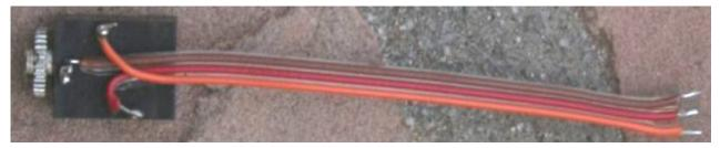
Figure 49. Use Brown/Red/Orange wire and connect up the headphone jack in the color order shown
