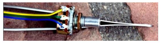
Figure 53. Use Yellow/Green/Blue wire to connect to R77, the 5K volume control pot in the color order shown
