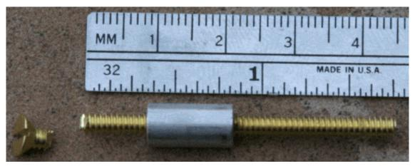
Figure 77. 2" brass screw cut back to a total length of 1 <sup>3</sup>/<sub>4</sub> inches.
