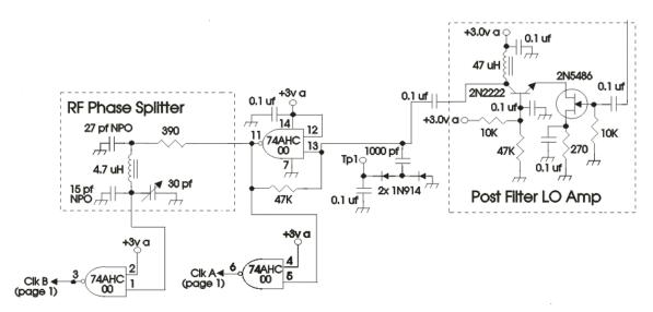
Figure 138. Schematic of LO amplifier and detector clock phase splitter
