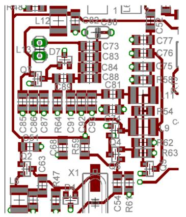
Figure 66. Close up of the PTO and Mixer section of the board
