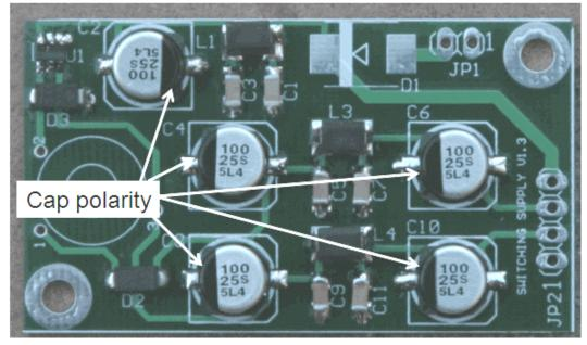
Figure 16. PS and Electrolytic Caps Polarity Details
