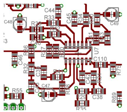
Figure 92. Close up of the 750 Hz Audio LPF section
