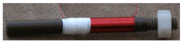
Figure 75. Coil with completed 105 turns. Turns wound tight and "shoulder to shoulder".
