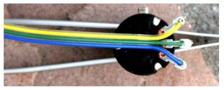
Figure 51. Use Yellow/Green/Blue wire to connect to R83, the 50k SCAF pot in the color order shown
