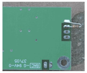
Figure 22. 3v Temporary 100 Ohm Load Resistor Connected to Bottom of Board
