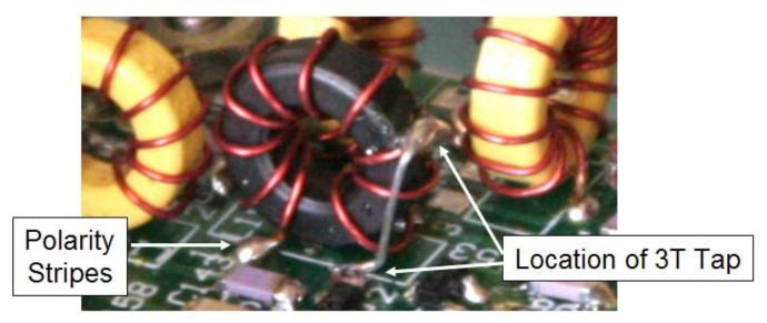
Figure 97. L19 mounted. 3T tap location shown.
