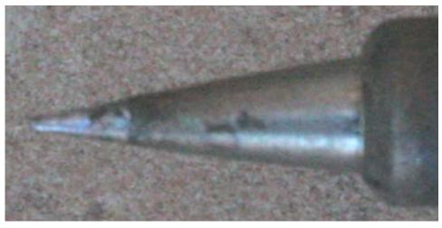
Figure 3. A very pointed soldering iron tip is a very big help for small surface mounted components
