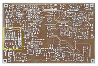
Figure 65. Board Location of the LO mixer and PTO circuitry
