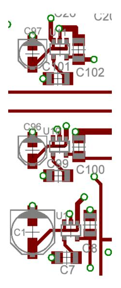
Figure 29. Location of the one 3v and two 5v LDO regulator sections
