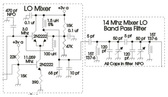
Figure 137. LO Mixer and IF Filter schematic
