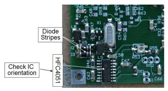
Figure 58. Proper orientation of U8, D2, and D3
