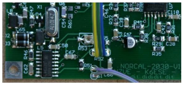
Figure 60. Connect the 25K RIT pot to the R52 header in the color order shown. Also attach a SPDT switch to S1
