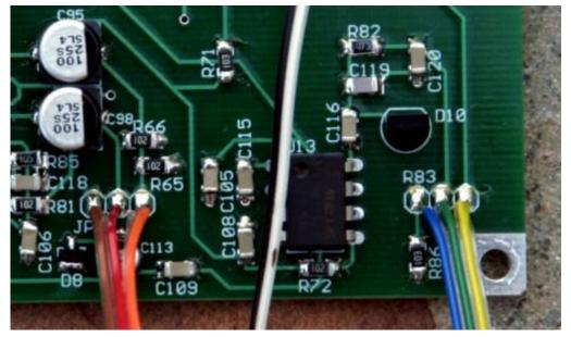
Figure 52. Connect the 50K SCAF pot to the R83 header pads in the color order shown
