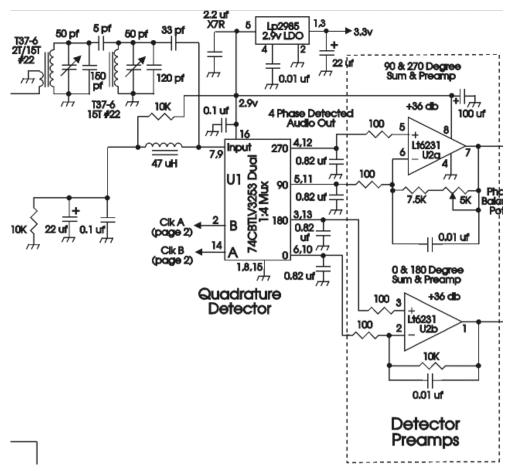
Figure 130. Tayloe quadrature detector and I/Q audio preamplifier schematic
