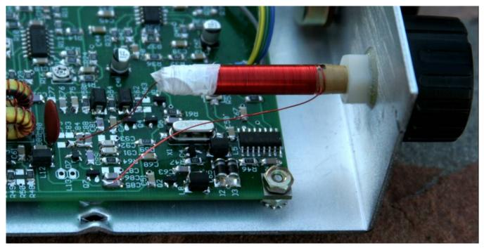
Figure 123. L13 PTO tuning coil as mounted. Remove turns off the end simply by pulling on the wire.
