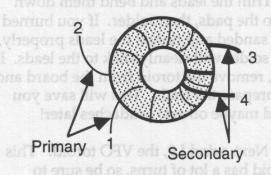
[] Remove the insulation from T1's leads as described above and install it on the circuit board. Make sure that the primary and secondary leads line up with the numbers on the PCB outline. Solder T1.
