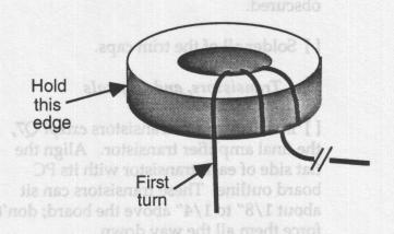
After winding, the turns should be spaced evenly around most of the core, leaving a small gap between the first and last turns as shown below. (Note that the number of turns shown in the drawing is different from the actual number of turns used.)
