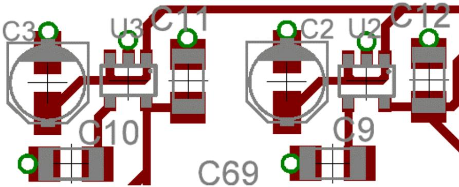
Figure 27. Close up of first two 3v LDO regulators
