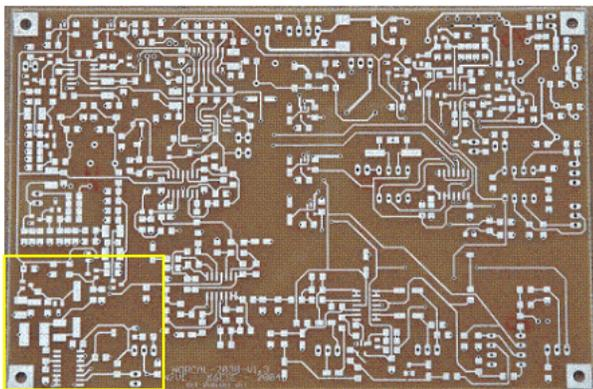
Figure 56. Location of VXO and T/R offset circuit.
