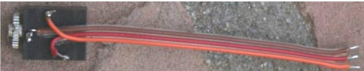
Figure 47. Use Brown/Red/Orange wire and connect up the paddle jack in the color order shown.
