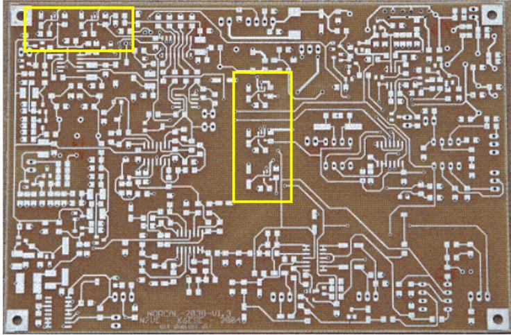
Figure 26. Location of the two 3v and 5v regulator sections
