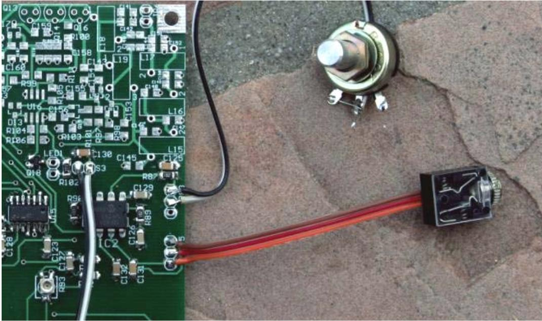
**Figure 48. Attach paddle jack to JP5 using the color order shown**
