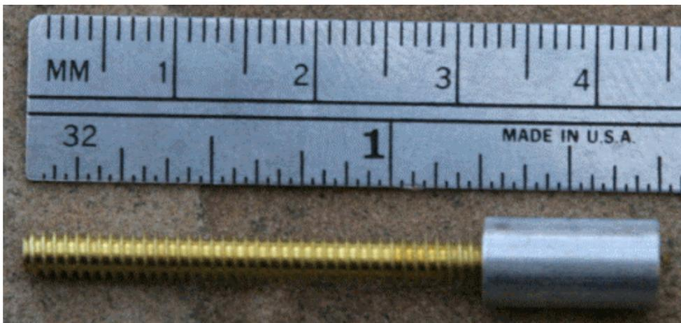
Figure 78. Final screw with mounted spacer.
