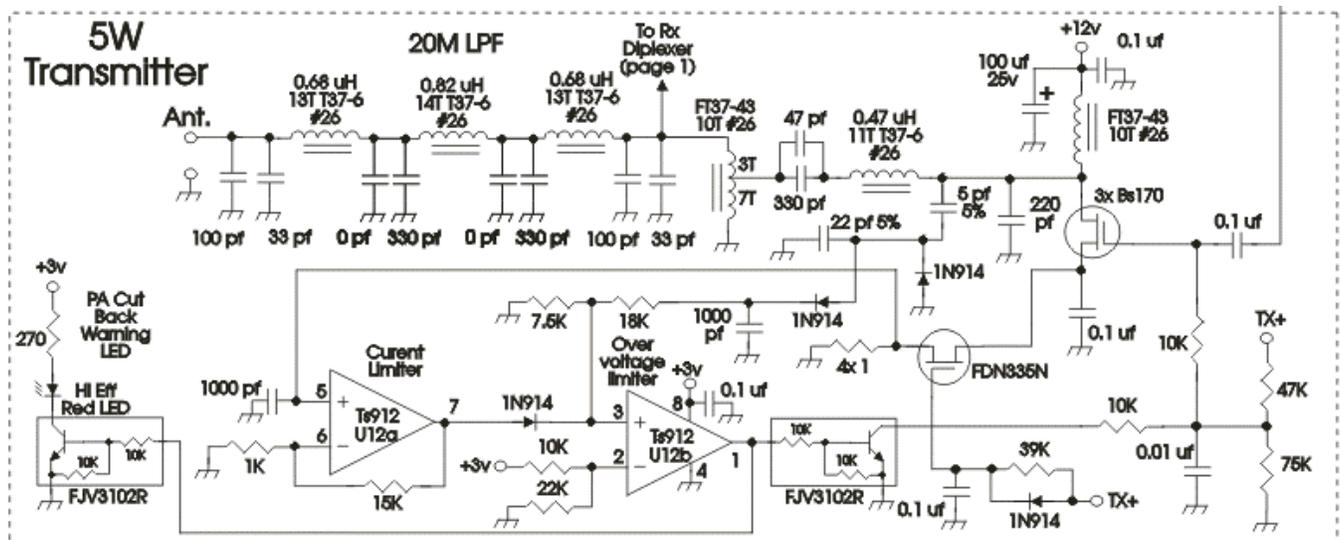
Figure 139. Schematic of Class E Transmitter
