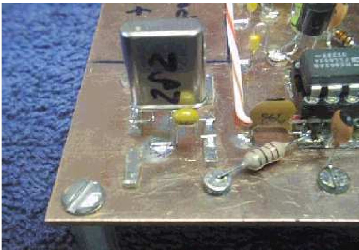
Fig. 23 Crystal Filter - Step 1, Another View
