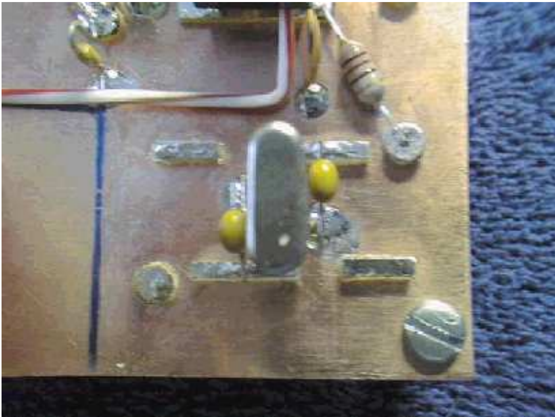
Fig. 24 Crystal Filter Step 1 Viewed from Above
